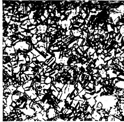
FIGURE 481. Metallographic structure of an annealed silicon bronze. Etched with \text{NH}_4\text{OH} + \text{H}_2\text{O}_2 . \times 75 . (Photomicrograph courtesy Research Department, Chase Brass & Copper Co.)
